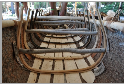
Figure 6. Carving canoe a thwart utilizing white cedar. Photo: Finney K., Great Lakes Lifeway Institute
